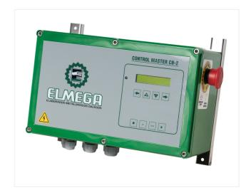
The CONTROL MASTER CB2 is an electrical panel that adapts to any of the winches manufactured by ELMEGA. Its features include ease of use, possibility of manual or scheduled use, winter operating mode, obstacle detection or operating history, among others.
