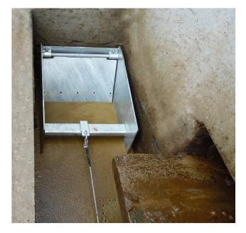
These scrapers are specially designed to clean and discharge slurry channels.
