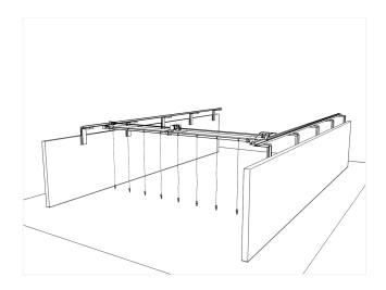
This cow herder is supplied with a rack and toothed wheels to achieve a completely parallel advance of its two ends. It is adjustable from 5 to 6m to adapt to conventional spinach sauces and those of 60°. It consists of double motorization, one for the longitudinal advance of the pusher and another for the curtain, allowing to lot groups of animals.
