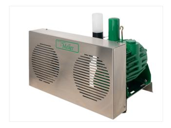
These long-proven depressor units are characterized by their performance, durability and high quality and finish. They are lubricated with SAE 10 oil. These depresser units include: vacuum pump, pulley, grease nipple, silencer, non-return valve, stainless steel base with belt tensioner, stainless steel belt protection, and vacuum tank. They can be supplied with or without motor and with a plastic or stainless steel vacuum tank according to the customer's preferences.
